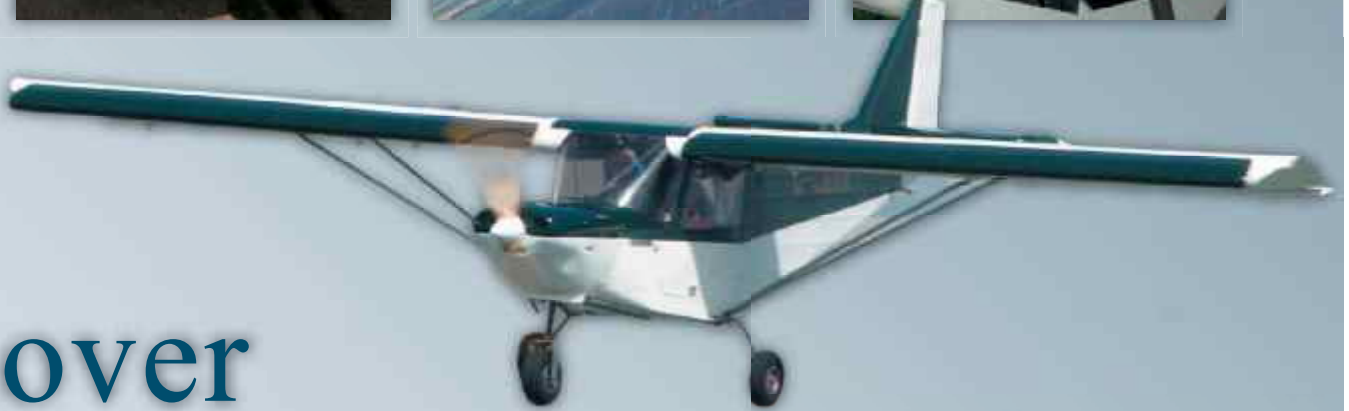
Flat skins relieved with creases to help reduce drumming.
